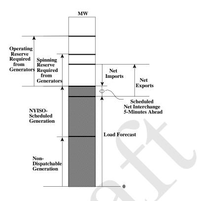
Figure 6-2 Control Area Constraints
