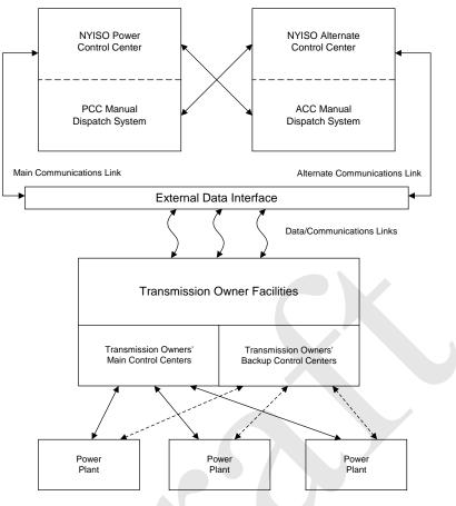
Figure 2-4 Backup Operations Configuration
